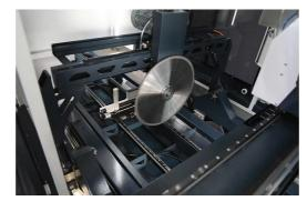
profiles, even hard steel and stainless steel profiles. The cutting unit that is placed at the back of the bridge can cut the profiles into 90, 45 and 135 degrees automatically without moving the profiles away from the machine. The saw blade moves in a radial way to cut the profiles. This machine is designed especially for large sliding windows that have large frame profiles to cut.
